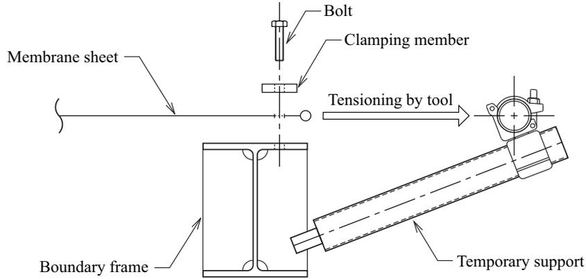
Figure 2: Construction process of a frame-supported membrane structure.
