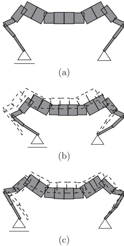
Figure 14: Optimal solution of Type 2 for Problem P6 under stress constraints; (a) undeformed shape, (b) deformed shape magnified by 10 under  $P_1$ ; dotted line: undeformed shape, (c) deformed shape magnified by 10 under  $P_2$  after constraining node 2; dotted line: undeformed shape.
