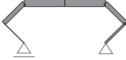
Figure 13: Optimal solution of Type 2 for Problem P5 under displacement constraint.
