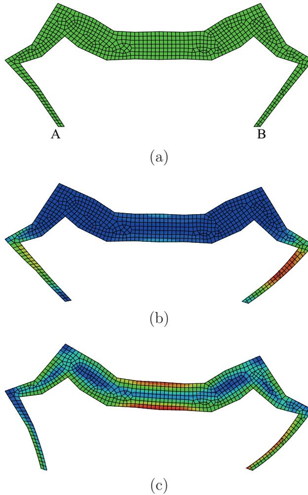
Figure 16: Deformation and contour lines of von Mises stress by FE-analysis for verification of optimal solution of Type 2; (a) undeformed shape, (b) deformed shape magnified by 10 under  $P_1$ , (c) deformed shape magnified by 10 under  $P_2$  after constraining node 2.
