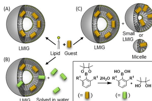
**Scheme 2** Schematic illustration of (A) stable LMIG [category (i)], (B) the dissolution of the guest molecules released from LMIG in water [category (ii)] and (C) the formation of small aggregates between the guest molecules released from LMIG and the lipids [category (iii)].
