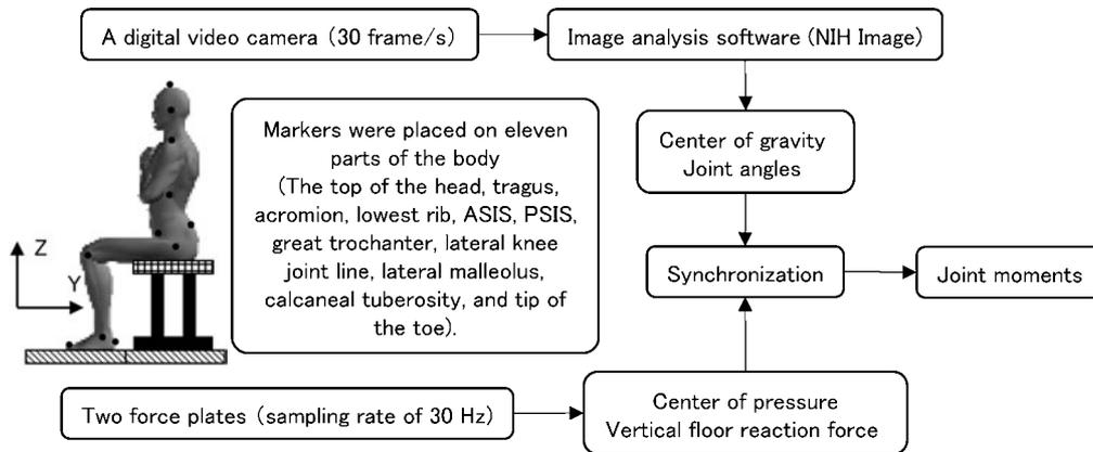
Fig. 1. Measurement system.
