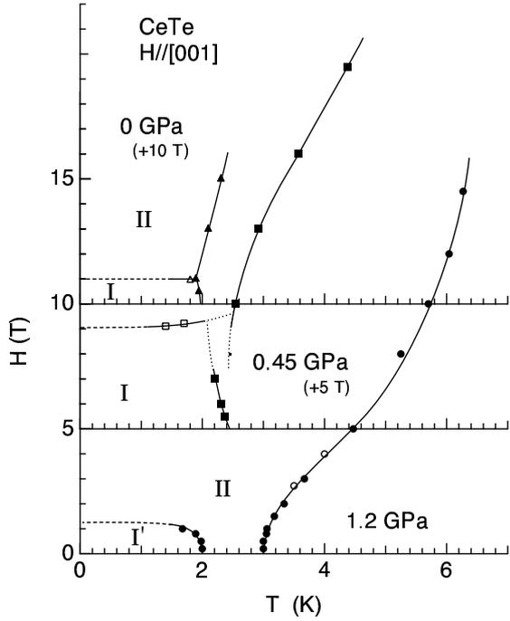
Fig. 3. Magnetic phase diagram of CeTe under high pressures. Solid and open symbols are from  $M(T)$  and  $M(H)$  measurements, respectively. The vertical axes for 0 GPa and 0.45 GPa are shifted by 10 T and 5 T, respectively. The lines are guides for the eye. The dashed lines are speculations to  $T=0$ . The dotted lines for 0.45 GPa are the obscure boundaries that were difficult to determine unambiguously.
