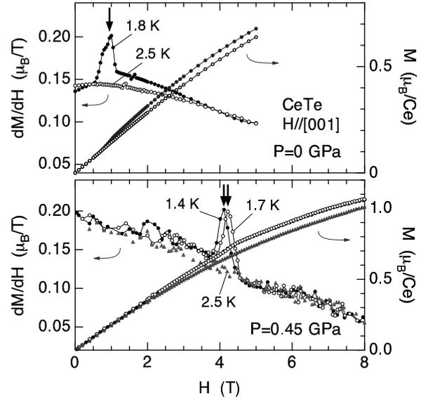
Fig. 4. Magnetic-field dependences of magnetization and their field derivatives. The  $M(H)$  curves were measured in the SQUID magnetometer for  $P=0$  GPa and in the 15 T magnet for  $P=0.45$  GPa, respectively. The arrows on the peaks in  $dM/dH$  represent the phase boundaries plotted in Fig. 3.
