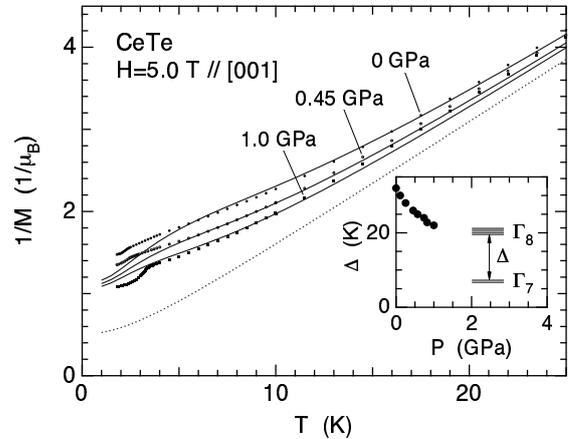
Fig. 5. Temperature dependences of inverse magnetization at  $H=5$  T. The solid lines are the calculated curves described in the text. The dotted line is for a free ion without CEF. The inset shows the pressure dependence of the CEF splitting obtained from the fitting.
