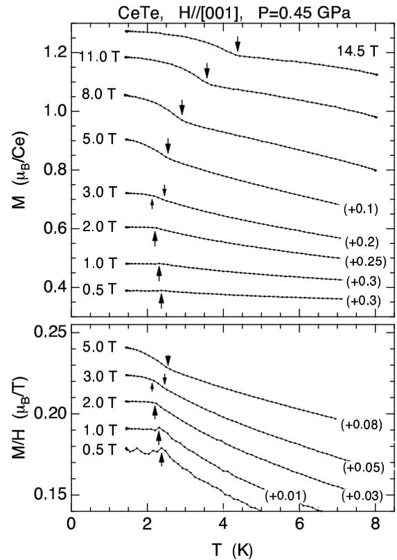
Fig. 2. Temperature dependence of magnetization under high pressure of 0.45 GPa. Arrows indicate the transition temperatures. Low field region is shown in the bottom figure in the form of  $M/H$  with vertical shifts indicated in the parentheses.
