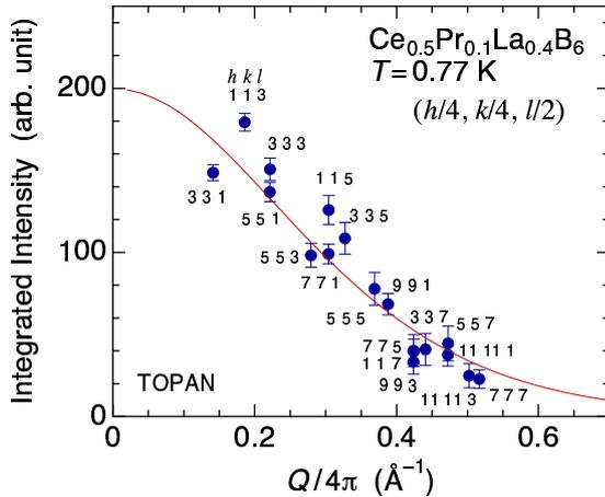
Fig. 4. (Color online)  $Q$  dependence of the Lorentz-factor-corrected intensities of the  $(\frac{1}{4}, \frac{1}{4}, \frac{1}{2})$ -equivalent reflections. The solid line shows  $|f(Q)|^2$  in the dipole approximation averaged for the Ce and Pr compositions.
