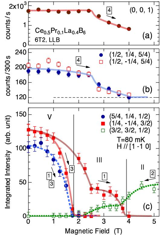
Fig. 5. (Color online) Magnetic field dependences of the intensities of the (a)  $(0, 0, 1)$  nuclear peak, (b)  $(\frac{1}{2}, \frac{1}{4}, \frac{5}{4})$  and  $(\frac{1}{2}, -\frac{1}{4}, \frac{5}{4})$  magnetic peaks, and (c)  $(\frac{5}{4}, \frac{1}{4}, \frac{1}{2})$ ,  $(\frac{1}{4}, -\frac{1}{4}, \frac{3}{2})$ , and  $(\frac{3}{2}, \frac{3}{2}, \frac{1}{2})$  magnetic peaks. The numbers in the square boxes represent the sequence of the scans. The solid and dashed lines are visual guides.
