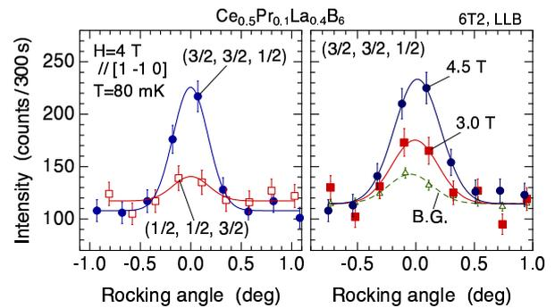
Fig. 6. (Color online) Rocking scans of the  $(\frac{3}{2}, \frac{3}{2}, \frac{1}{2})$  and  $(\frac{1}{2}, \frac{1}{2}, \frac{3}{2})$  reflections in magnetic fields. B.G. represents the background for  $(\frac{3}{2}, \frac{3}{2}, \frac{1}{2})$  due to the  $\lambda/2$  contamination in the incident beam, which is not detected for  $(\frac{1}{2}, \frac{1}{2}, \frac{3}{2})$ .
