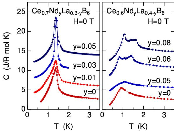
Fig. 8. (Color online) Specific heat of  $Ce_xNd_yLa_{1-x-y}B_6$ . Data for  $y > 0$  are shifted.
