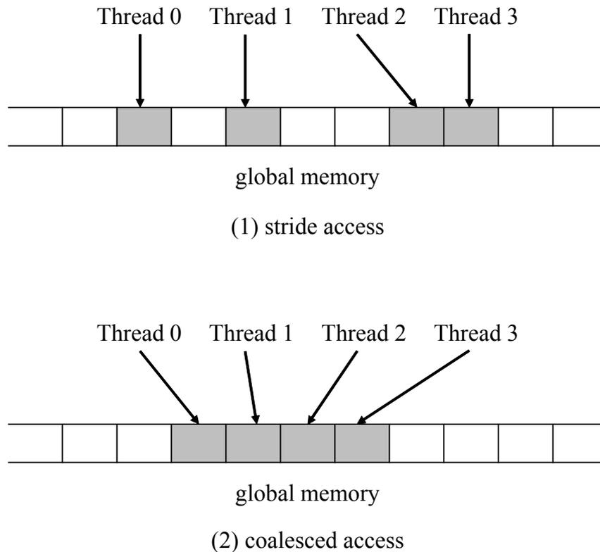
Figure 2.3: Stride access and coalesced access to the global memory
