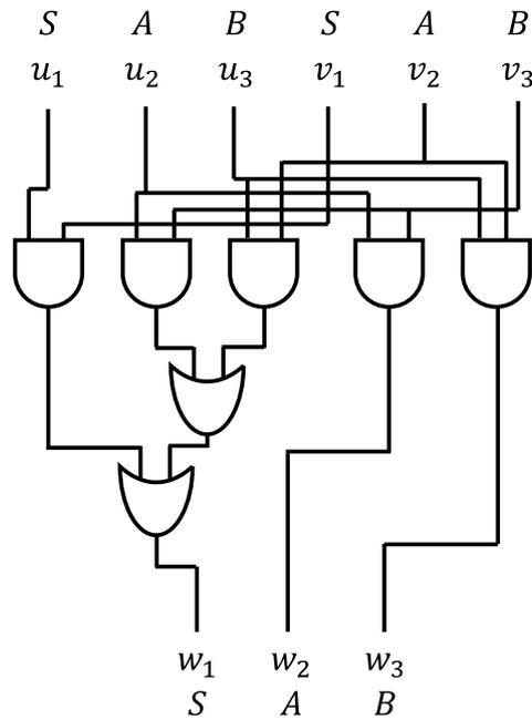
Figure 7.2: The circuit for computing  $\otimes_{G_{\text{example}}}$
