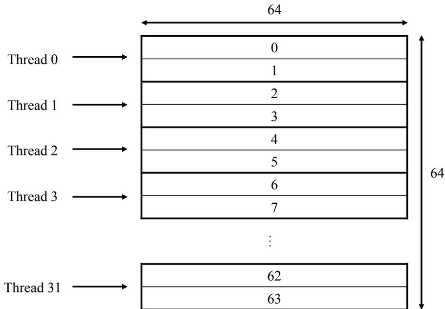
Figure 6.6: Words accessed by threads executing Algorithm DOUBLE-WORD
