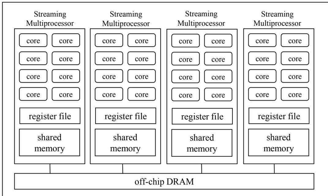
Figure 2.1: GPU architecture
