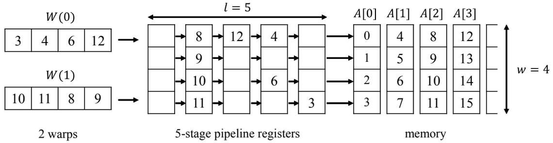
Figure 3.1: The UMM with width  $w = 4$  and latency  $l = 5$
