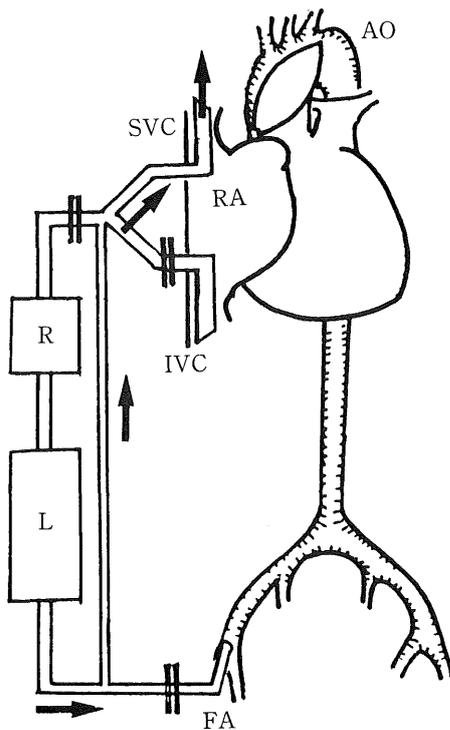
**Fig. 1.** Perfusion circuit during retrograde cerebral perfusion
