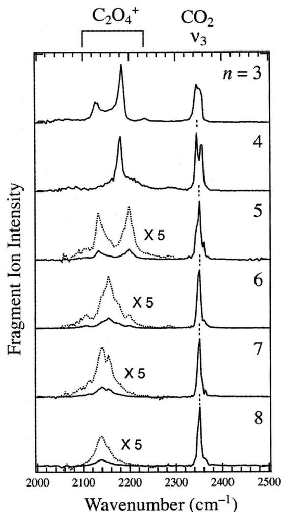
FIG. 2. Expanded views of the IRPD spectra of  $(\text{CO}_2)_n^+$  with  $n=3-8$  in the  $2000-2500 \text{ cm}^{-1}$  region. Intensity of the fragment ion for each spectrum is normalized with the maximum value in this region.
