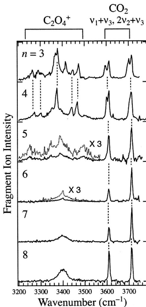
FIG. 4. Expanded views of the IRPD spectra of  $(\text{CO}_2)_n^+$  with  $n=3-8$  in the 3200–3750  $\text{cm}^{-1}$  region. Intensity of the fragment ion for each spectrum is normalized with the maximum value in this region.
