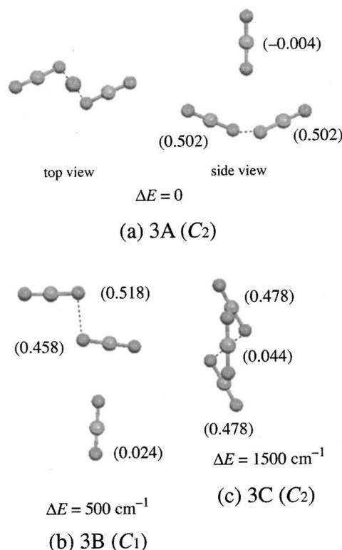
FIG. 7. Optimized structures of  $(CO_2)_3^+$  calculated at the MP2/6-311+G\* level. Numbers in parentheses represent the positive charge distribution on the constituent  $CO_2$  molecules.
