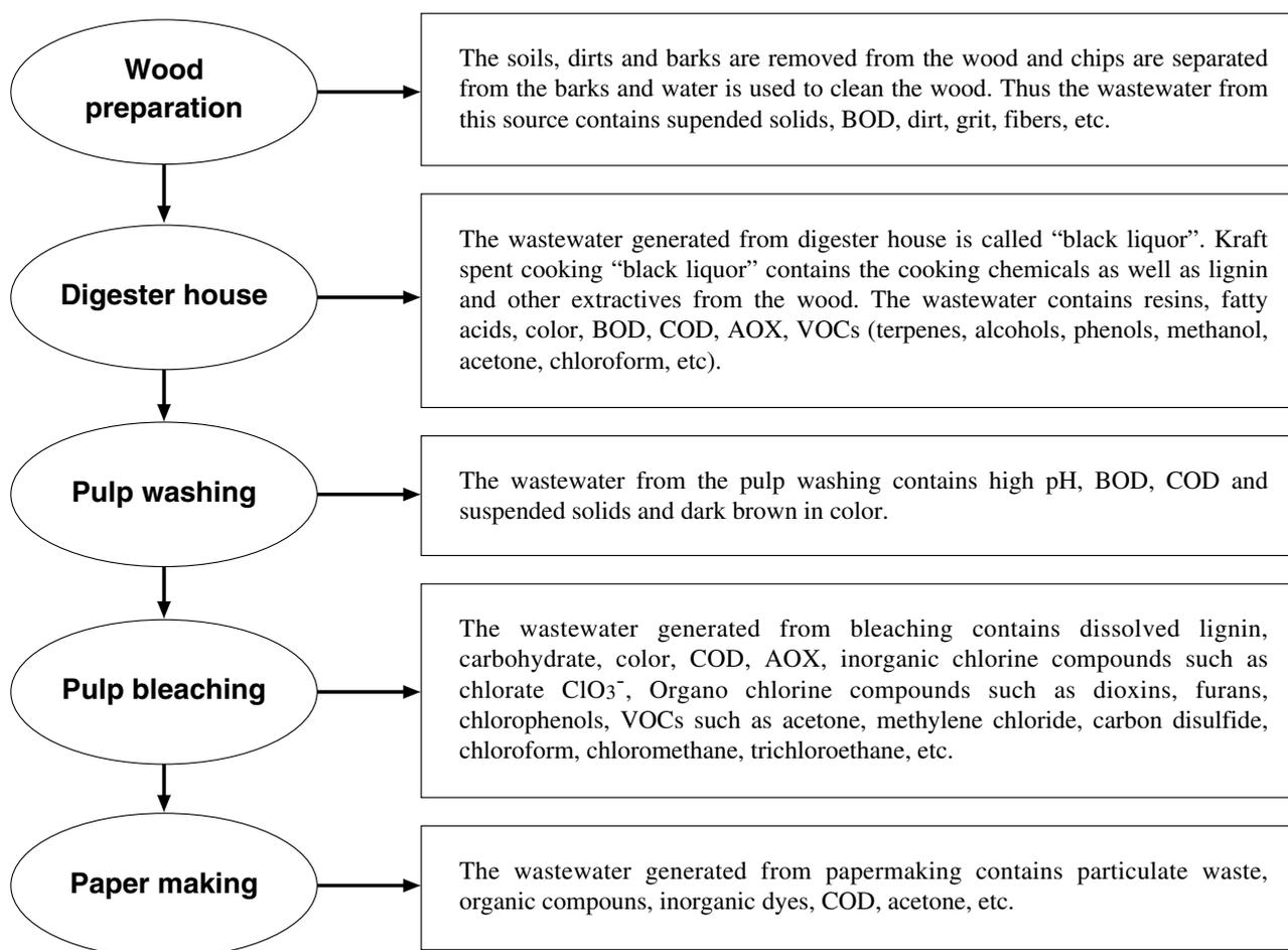
**Figure 1.** Process for preparation of pulp and paper from woody and non-woody plants, and generation of pollutants from various sources of pulping and paper making.
