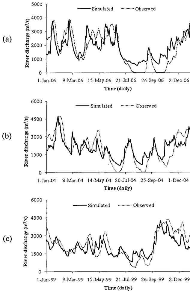
**Figure 9:** Hydrograph (observed vs. simulated) of Kapuas River in Sanggau outlet in 2006 (a), 2004 (b), and 1999 (c).
