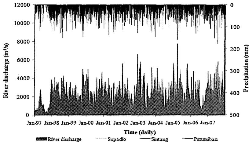
**Figure 11:** Simulated Kapuas River discharge and daily precipitation in Supadio, Sintang and Putussibau meteorological stations.
