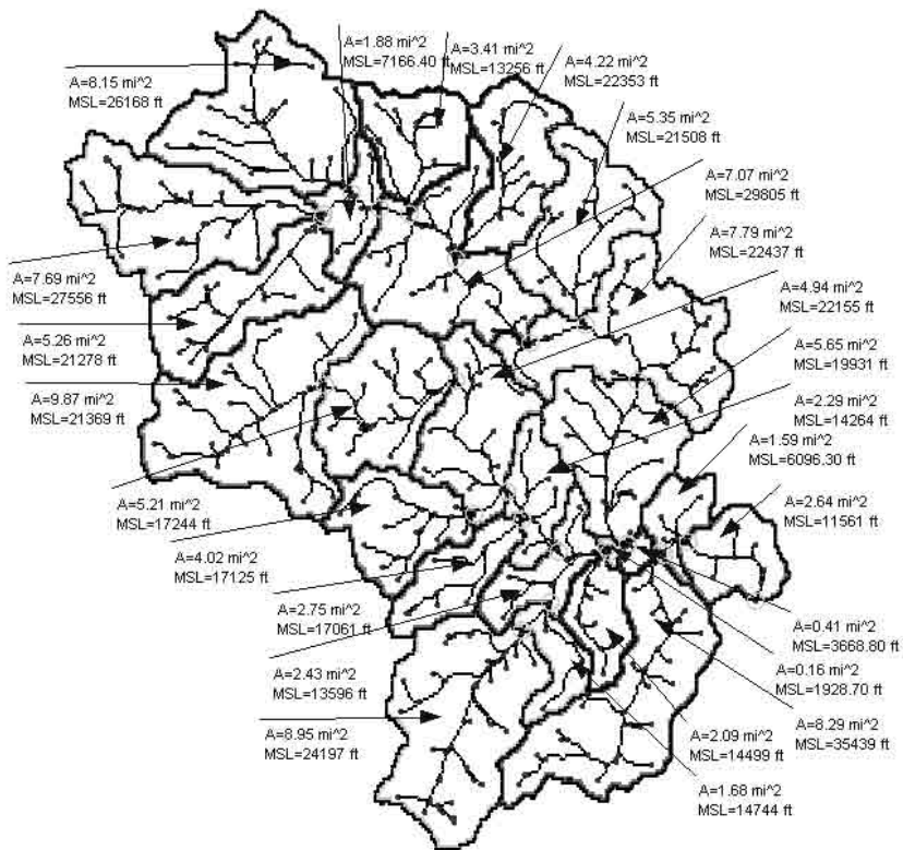
Figure 3: Haji dam watershed with its sub-watersheds and stream network; also is presented information about area for each sub-watershed (A) and stream length (MSL).
