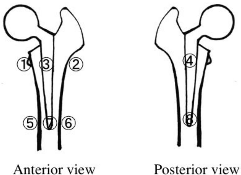
Fig. 4. Sites of attachment of strain gauges.
