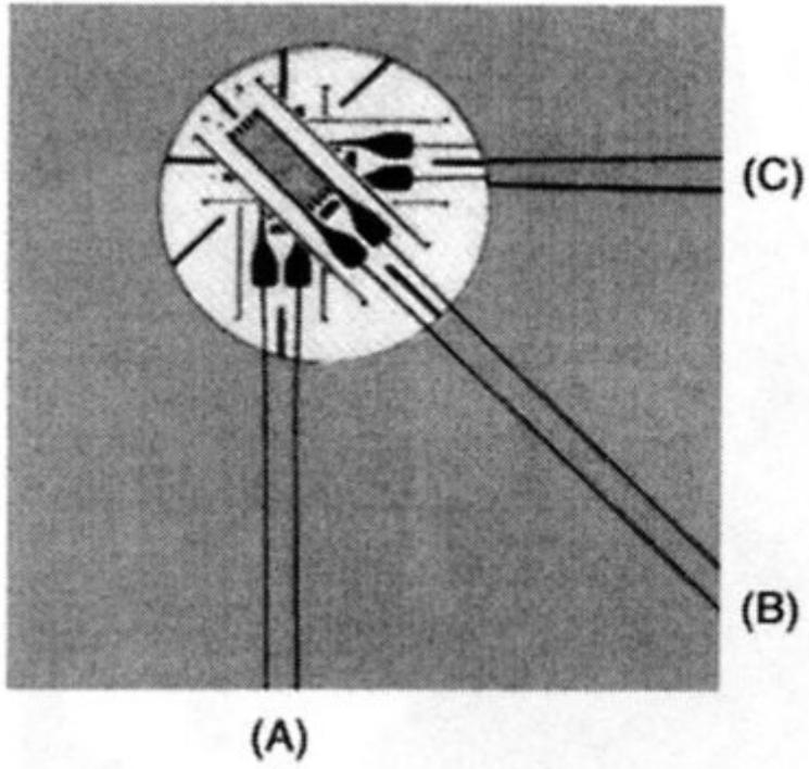
Fig. 3. Strain gauge; gauge element a (A), gauge element b (B), gauge element c (C)
