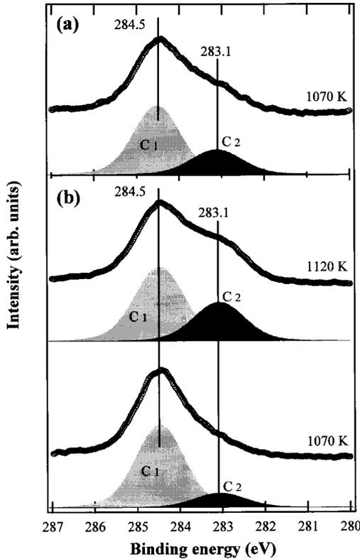
FIG. 4. C 1s core level spectrum measured after annealing the 1.0-ML film adsorbed on a Si(001)-(2 $\times$ 1) surface at 1070 K (a), and those after annealing the C<sub>60</sub> film adsorbed on a Si(111)-(7 $\times$ 7) surface at 1070 and 1120 K (b). The open circles are the experimental data, and the solid lines overlapped with open circles are the fitting curves. Each hatching indicates a different C 1s component.
