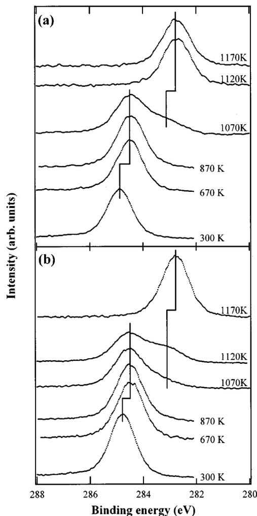
FIG. 3. Temperature-dependent C 1s spectra of the 1.0-ML  $C_{60}$  film adsorbed on Si(001)- $(2 \times 1)$  (a) and Si(111)- $(7 \times 7)$  (b) surfaces, observed by the Mg  $K\alpha$  line. The temperatures are 300, 670, 870, 1070, 1120, and 1170 K in both (a) and (b).
