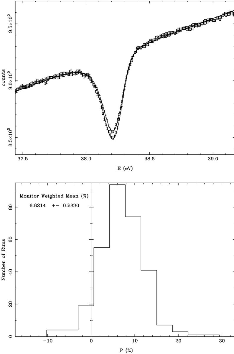
FIG. 3. (top)  $^{232}\text{Th}$  transmission spectra for two helicity states near the 38.2-eV resonance. (bottom) Histogram of the asymmetries obtained for each of 150 runs for the resonance shown at the top of the figure.
