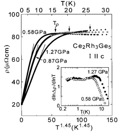
FIG. 4. Resistivity of  $\text{Ce}_2\text{Rh}_3\text{Ge}_5$  along the  $c$  axis as a function of  $T^{1.45}$  under various pressures above 0.58 GPa. Here  $T_\rho$  is the temperature where the resistivity exhibits a maximum or shoulder. The inset shows the temperature dependence of  $d \ln \Delta\rho / d \ln T$ , where  $\Delta\rho = \rho - \rho_0$ , at 0.58 and 1.27 GPa.
