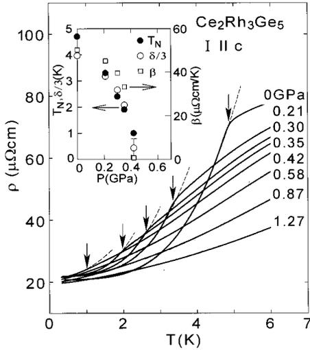
FIG. 3. Low-temperature resistivity of  $\text{Ce}_2\text{Rh}_3\text{Ge}_5$  along the  $c$  axis for several pressures. The dashed lines are the fits by Eq. (2) given in the text. The inset shows the pressure dependence of the antiferromagnetic ordering temperature  $T_N$ , the spin-wave scattering weight  $\beta$ , and the spin-wave energy gap  $\delta$  (see text).
