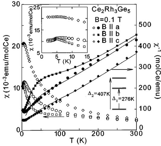
FIG. 1. Temperature dependence of magnetic susceptibility  $\chi(T)$  and its inverse along the three principal axes of  $\text{Ce}_2\text{Rh}_3\text{Ge}_5$ . The solid lines and the level scheme show the results calculated with a crystal-field model. The inset shows  $\chi(T)$  below 15 K.
