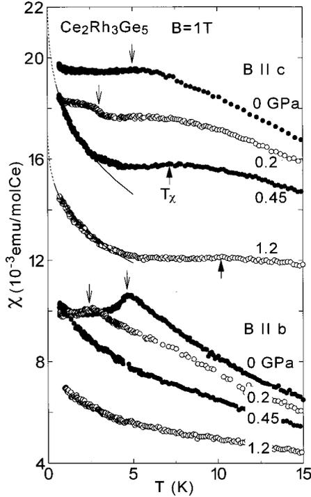
FIG. 6. Temperature variations of magnetic susceptibility of  $\text{Ce}_2\text{Rh}_3\text{Ge}_5$  for  $B\parallel b$  and  $B\parallel c$  below 15 K under pressure. The solid lines represent the fit with  $\chi(T) = \chi_0 - DT^m$ .
