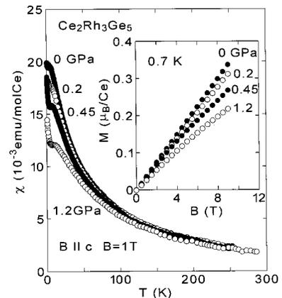
FIG. 5. Temperature dependence of magnetic susceptibility of  $\text{Ce}_2\text{Rh}_3\text{Ge}_5$  for  $B \parallel c$  under various pressures. The inset shows the isothermal magnetization curves at 0.7 K under pressure.
