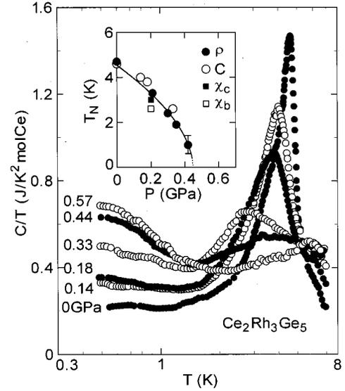
FIG. 7. Specific heat divided by temperature  $C/T$  as a function of  $T$  for  $\text{Ce}_2\text{Rh}_3\text{Ge}_5$  under various pressures. The inset shows the pressure dependence of magnetic transition temperature  $T_N$ .
