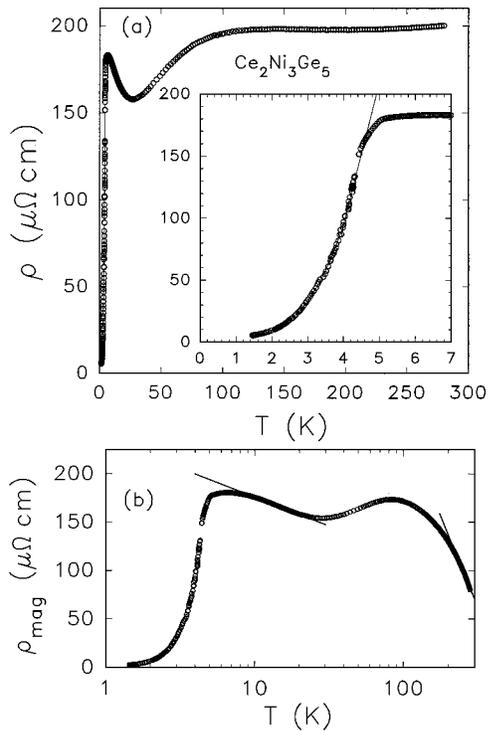
FIG. 2. (a) Electrical resistivity of  $\text{Ce}_2\text{Ni}_3\text{Ge}_5$  in the temperature interval 1.3–300 K. The inset shows an expanded view of the low-temperature part of the resistivity. The solid line is the fit to the data below 4 K (see text). (b) Magnetic contribution to the electrical resistivity  $\rho_{\text{mag}}$  vs  $\ln T$ .
