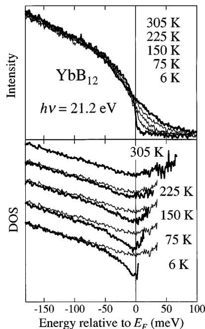
FIG. 3. Top: High-resolution photoemission spectra of  $\text{YbB}_{12}$  near  $E_F$  ( $h\nu = 21.2$  eV). Bottom: Spectral DOS at each temperature (thick curve) together with the DOS at 305 K (thin curve). The bottom line is the zero for the DOS at 6 K and the other densities of states have been offset.
