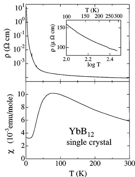
FIG. 1. Electrical resistivity and magnetic susceptibility of the  $\text{YbB}_{12}$  single crystal used in the present work. High-temperature ( $100 < T < 300$  K) resistivity is plotted in the inset.
