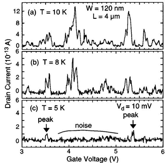
FIG. 5.  $I_d$  vs  $V_g$  characteristics at three different temperatures: (a)  $T = 10$  K, (b)  $T = 8$  K, (c)  $T = 5$  K.  $V_d$  is 10 mV. The nominal wire length and width are 4  $\mu\text{m}$  and 120 nm, respectively. The average thickness of the poly-Si wire is  $\sim 7$  nm.
