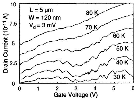
FIG. 8.  $I_d$  vs  $V_g$  characteristics of poly-Si wire at  $V_d=3$  mV for various temperatures from 30 to 80 K. The conductance oscillations are observed up to about 80 K. The nominal wire length and width are 5  $\mu\text{m}$  and 120 nm, respectively. The average thickness of the poly-Si wire is  $\sim 7$  nm.
