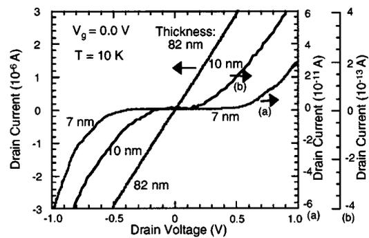
FIG. 2. Drain current ( $I_d$ ) vs drain voltage ( $V_d$ ) characteristics for three samples with different poly-Si thicknesses. Gate voltage  $V_g$  is 0.0 V. The measurement temperature is 10 K. The nominal length (5  $\mu\text{m}$ ) and width (100 nm) of the three samples are almost constant. The average thicknesses of the three samples are  $\sim 7$  nm (from 4 to 9 nm),  $\sim 10$  nm (from 8 to 12 nm), and  $\sim 82$  nm (from 80 to 86 nm).
