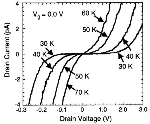
FIG. 7.  $I_d$  vs  $V_d$  characteristics at four different temperatures.  $V_g$  is 0.0 V. The nominal wire length and width are 7  $\mu\text{m}$  and 120 nm, respectively. The average thickness of the poly-Si wire is  $\sim 7$  nm.
