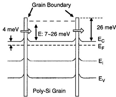
FIG. 10. Proposed energy-band diagram for the smallest island in the poly-Si wire.  $E$  is the energy level when one electron is added to the island.
