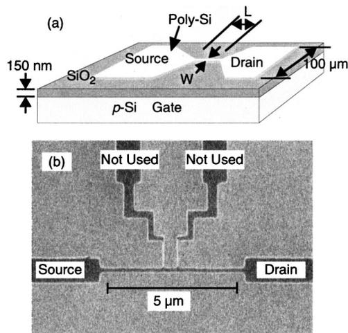
FIG. 1. (a) Schematic diagram of fabricated transistor structure with a narrow, extremely thin poly-Si wire. The average sample thicknesses are  $\sim 7$ ,  $\sim 10$ , and  $\sim 82$  nm. The nominal wire length  $L$  and the width  $W$  of the fabricated pattern are 4, 5, and 7  $\mu\text{m}$  and 95–2000 nm, respectively. (b) Plan-view SEM of the fabricated poly-Si wire. The wire length and the width are 5  $\mu\text{m}$  and 175 nm, respectively.
