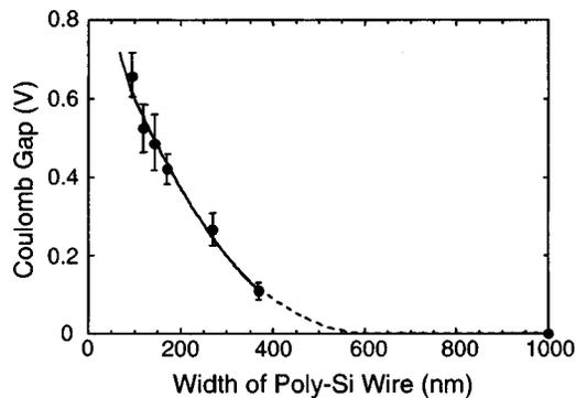
FIG. 12. Wire width dependence of Coulomb gap at 5 K. The length of the measured wires is constant ( $7 \mu\text{m}$ ). The average thickness of the poly-Si wires is constant ( $\sim 7 \text{ nm}$ ).
