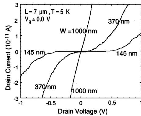
FIG. 11. Wire width dependence of  $I_d$  vs  $V_d$  characteristics at 5 K.  $V_g$  is 0.0 V. The length of the measured wires is constant (7  $\mu\text{m}$ ). The average thickness of the poly-Si wires is constant ( $\sim 7$  nm).
