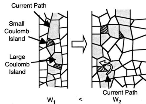
FIG. 13. Schematic representation of the wire dependence of the conduction mechanism.
