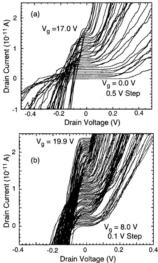
FIG. 4.  $I_d$  vs  $V_d$  characteristics as a function of substrate voltage ( $V_g$ ) at 6 K (a)  $V_g$  from 0.0 to 17.0 V in  $V_g$  steps of 0.5 V. Each curve is offset by 0.5 pA of  $I_d$  for clarity. (b)  $V_g$  from 8.0 to 19.9 V in  $V_g$  steps of 0.1 V. Each curve is offset by 0.2 pA. The nominal wire length and width are 5  $\mu\text{m}$  and 170 nm, respectively. The average thickness of the poly-Si wire is  $\sim 7$  nm.
