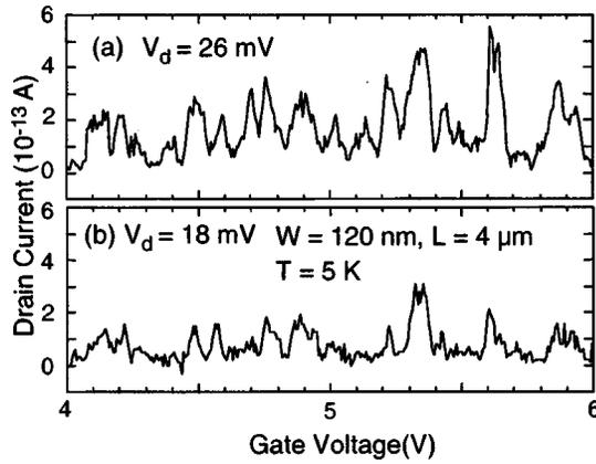
FIG. 6.  $I_d$  vs  $V_g$  characteristics at two different drain voltages: (a)  $V_d = 26$  mV and (b)  $V_d = 18$  mV. The graph for  $V_d = 10$  mV is the same as that shown in Fig. 5(c). The measurement temperature was 5 K. The nominal wire length and width are 4  $\mu\text{m}$  and 120 nm, respectively. The average thickness of the poly-Si wire is  $\sim 7$  nm.
