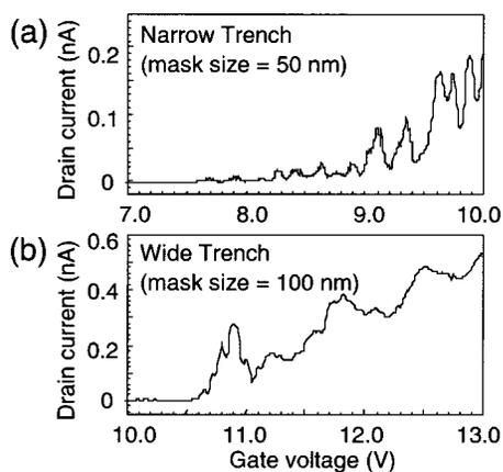
FIG. 4. Drain current ( $I_d$ ) vs gate voltage ( $V_g$ ) characteristics of the single-electron transistor having different trench widths at 4.2 K. Drain voltage ( $V_{ds}$ ) is 1 mV. The mask size along the  $Y-Y'$  line in Fig. 1(a) is 100 nm. The width of the trench surface is estimated to be about 240 nm [(a), mask size of 50 nm] and 290 nm [(b), mask size of 100 nm] along the  $X-X'$  line.
