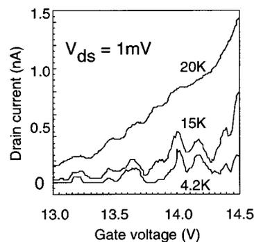
FIG. 3. Drain current ( $I_d$ ) vs gate voltage ( $V_g$ ) characteristics of the device (a) at 4.2, (b) at 15, and (c) at 20 K. Drain voltage ( $V_{ds}$ ) is 1 mV. The mask width of the trench [along the  $X-X'$  line in Fig. 1(a)] is 62.5 nm. The mask size along the  $Y-Y'$  line is 100 nm.
