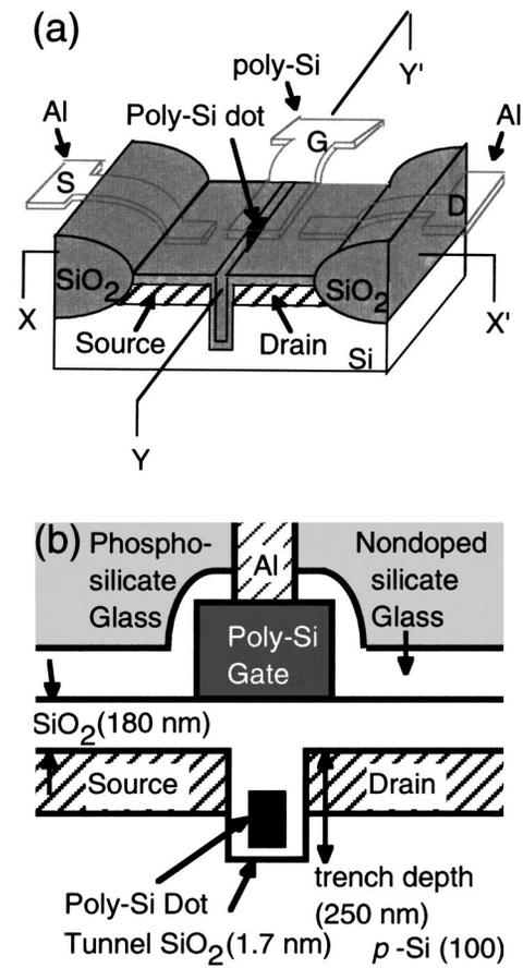
FIG. 1. (a) Schematic diagram of the Si single-electron transistor having double SiO<sub>2</sub> barriers with a poly-Si dot and (b) cross-sectional view along the X–X' line.
