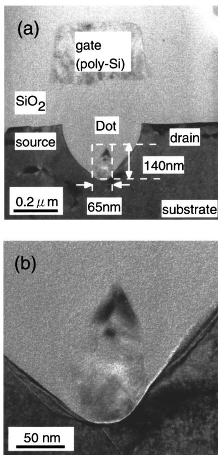
FIG. 2. (a) TEM micrograph of cross-sectional view along the  $X-X'$  line in Fig. 1 and (b) high-resolution micrograph.
