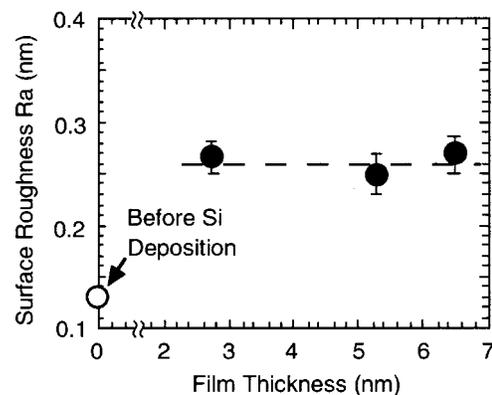
FIG. 5. Surface roughness vs film thickness. The substrate temperature at  $\text{Si}_2\text{H}_6$  exposure is fixed at  $355^\circ\text{C}$ . The gas exposure times are the same as in Fig. 4. It was confirmed that the film thickness was proportional to the growth cycle.
