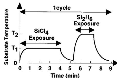
FIG. 1. Typical time sequence of gas supply and substrate temperature control.  $T_1$  and  $T_2$  indicate the substrate temperature during SiCl<sub>4</sub> exposure and Si<sub>2</sub>H<sub>6</sub> exposure, respectively. The substrate temperature was computer-controlled synchronized with the gas supply. The vacuum evacuation time between SiCl<sub>4</sub> and Si<sub>2</sub>H<sub>6</sub> exposures is 90 s. The pressure in the chamber just before each gas supply is  $\sim 2 \times 10^{-4}$  Torr.
