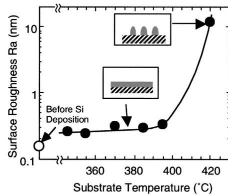
FIG. 4. Surface roughness vs substrate temperature at  $\text{Si}_2\text{H}_6$  exposure. The growth cycle is 20. The  $\text{SiCl}_4$  and  $\text{Si}_2\text{H}_6$  exposure times are 4 and 2 min, respectively.
