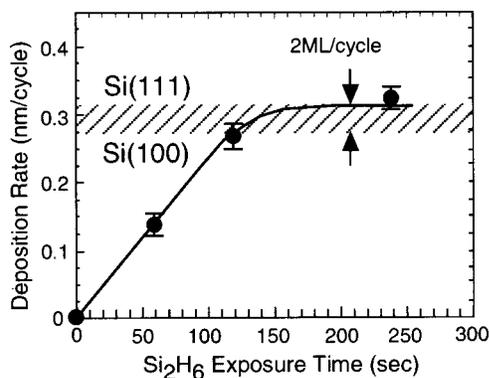
FIG. 3. Deposition rate of Si vs  $\text{Si}_2\text{H}_6$  exposure time at a substrate temperature of  $355^\circ\text{C}$ . The  $\text{SiCl}_4$  exposure time is fixed at 4 min.
