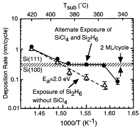
FIG. 2. Growth rate of Si as a function of substrate temperature at  $\text{Si}_2\text{H}_6$  exposure. The  $\text{SiCl}_4$  and  $\text{Si}_2\text{H}_6$  exposures times are 4 and 2 min, respectively. Two monolayer thicknesses of 0.27 nm for Si(100) and 0.31 nm for Si(111) are indicated in the figure.
