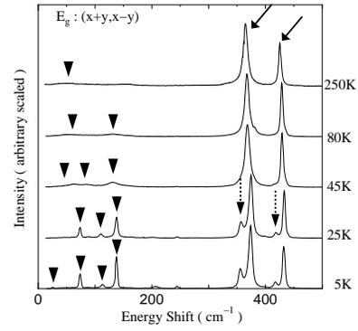
Fig. 1. Representative temperature dependence of  $E_g$  spectra of  $\text{PrRu}_4\text{P}_{12}$ . The solid arrows denote the Raman-active  $E_g$  phonons in the high temperature phase ( $\text{Im}\bar{3}$ ), and dotted arrows are phonons observed below  $T_{MI}$ . The triangles are CF excitations at the low energy region.
