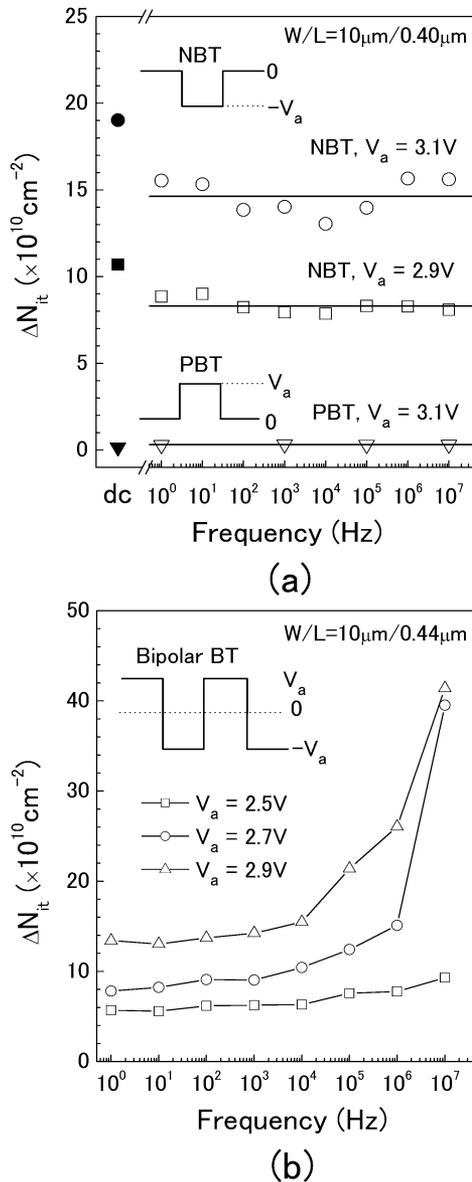
Fig. 1. Interface trap generation  $\Delta N_{it}$  as a function of stress frequency at different stress voltage  $V_{stress}$ , under (a) unipolar pulsed stress ( $L = 0.40 \mu\text{m}$ ), (b) bipolar pulsed stress ( $L = 0.44 \mu\text{m}$ ). Stressed at  $125^\circ\text{C}$  for  $10^3$  s. The data of dc stresses are also shown for comparison, whose nominal stress time is 500 s. Inset is a schematic waveform applied on the gate.
