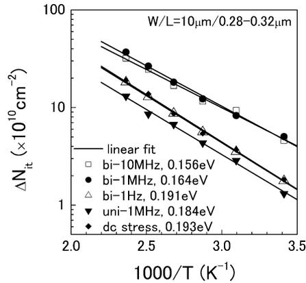
Fig. 4. Temperature dependence of  $\Delta N_{it}$  at five typical stress configurations. Devices with  $L = 0.28\text{--}0.32\ \mu\text{m}$ , stressed for  $10^3\ \text{s}$  at  $V_a = 2.9\ \text{V}$  except that  $V_a = 2.6\ \text{V}$  for 10-MHz bipolar stress to avoid  $\Delta N_{it}$  saturation. The activation energy  $E_a$  was extracted from the linear fitting of these Arrhenius plots.
