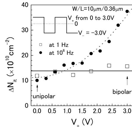
Fig. 2. Interface trap generation  $\Delta N_{it}$  under unsymmetrical bipolar BT stress as a function of  $V^+$  at 1 and  $10^6$  Hz.  $V_-$  is fixed to  $-3.0$  V. Devices with  $L = 0.36 \mu\text{m}$ , stressed at  $125^\circ\text{C}$  for  $10^3$  s. Inset is a schematic waveform applied on the gate.
