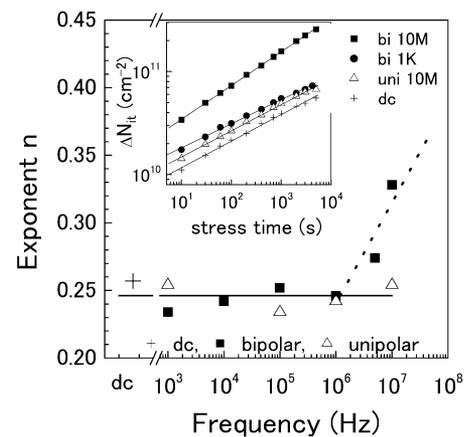
Fig. 3. Exponent  $n$  of the  $\Delta N_{it}$  time power function as a function of stress frequency at unipolar and bipolar pulsed stresses. The data of dc stress is also given for comparison. Inset is the time evolution of  $\Delta N_{it}$  for four typical stresses. The exponent  $n$  was extracted from the linear fitting of these plots.
