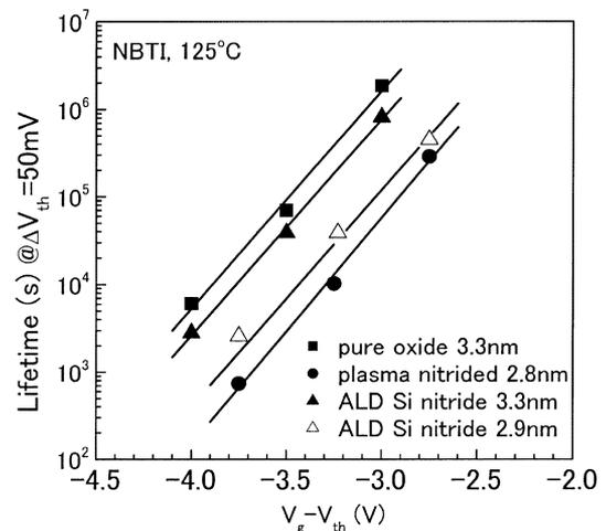
Fig. 3. Device lifetime as a function of  $V_g - V_{th}$  at 125 °C for peripheral pMOS transistors with  $L/W = 2 \mu\text{m}/10 \mu\text{m}$ .
