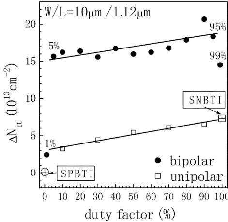
Fig. 2. Interface trap generation  $\Delta N_{it}$  as a function of duty factor under unipolar and bipolar stresses with a square waveform of  $t_R = t_F = 4.5$  ns and  $f = 10^6$  Hz. Devices have size of  $W/L = 10 \mu\text{m}/1.12 \mu\text{m}$  and are stressed at  $125^\circ\text{C}$  for  $10^3$  s. The 100% duty factor represents the dc negative BT stress (SNBTI), and the 0% duty factor represents the dc positive BT stress (SPBTI).
