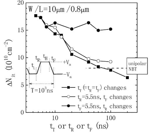
Fig. 3. Interface trap generation  $\Delta N_{it}$  as a function of  $t_R$  (or  $t_F$ ) under bipolar stresses at  $10^6$  Hz with a trapezoidal waveform. Inset shows a schematic waveform to define  $t_L$ ,  $t_R$ ,  $t_H$  and  $t_F$ . Devices have size of  $W/L = 10 \mu\text{m}/0.8 \mu\text{m}$  and are stressed at  $125^\circ\text{C}$  for  $10^3$  s. For comparison,  $\Delta N_{it}$  under unipolar stress with a square waveform ( $t_T = t_R = t_F = 4.5$  ns) is also shown.
