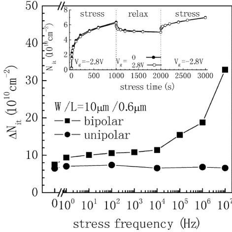
Fig. 1. Interface trap generation  $\Delta N_{it}$  as a function of stress frequency under unipolar and bipolar BT stresses with a square waveform of  $t_R = t_F = 4.5$  ns and duty factor of 50%. Devices have size of  $W/L = 10 \mu\text{m}/0.6 \mu\text{m}$  and are stressed at  $125^\circ\text{C}$  for  $10^3$  s. Inset is the time evolution of  $N_{it}$  under stress-relax-stress sequence.
