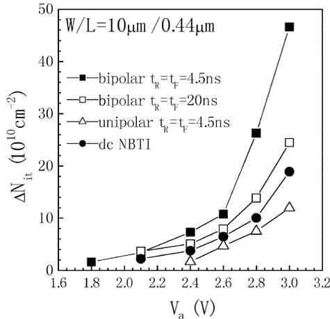
Fig. 4. Interface trap generation  $\Delta N_{it}$  as a function of  $V_a$  under bipolar, unipolar and dc NBT stresses. Devices have size of  $W/L = 10 \mu\text{m}/0.44 \mu\text{m}$  and are stressed at  $125^\circ\text{C}$  for  $10^3$  s. The dynamic stress has a square waveform of  $f = 10^6$  Hz,  $D = 50\%$ , and  $t_T = 4.5$  ns or 20 ns.
