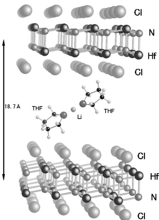
FIG. 1. Schematic structural model of  $\text{Li}_{0.48}(\text{THF})_y\text{HfNCl}$ .
