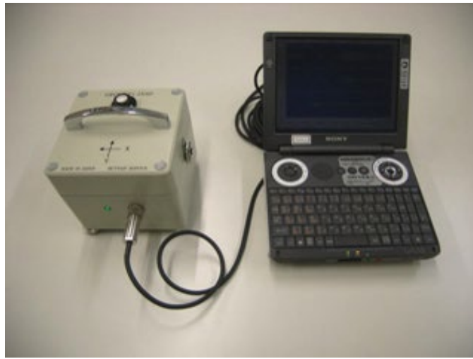
Figure 2-7. The GEODAQS-2S3D velocimeters developed by ANET Inc.
