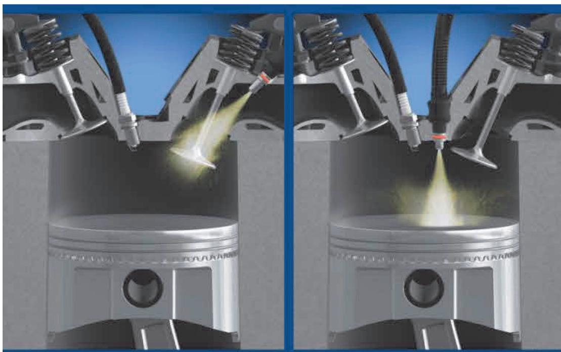
**(a) PFI engine****(b) DISI engine****Figure 1.6 PFI and DISI engine [17].**
