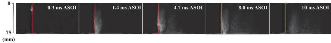
**Figure 3.4 Side view of wall-impingement spray**
