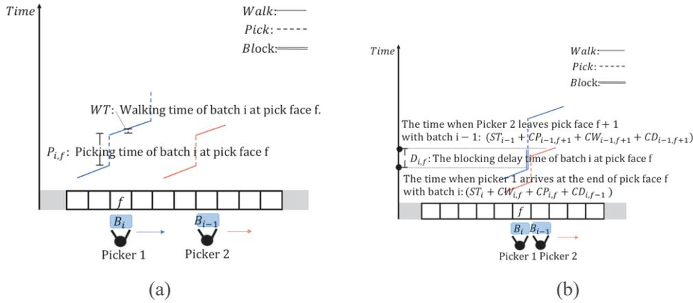
Figure 3-4 Time cost of pickers' behaviors in a picking line: (a) Picking and walking time; and (b) blocking delay time
