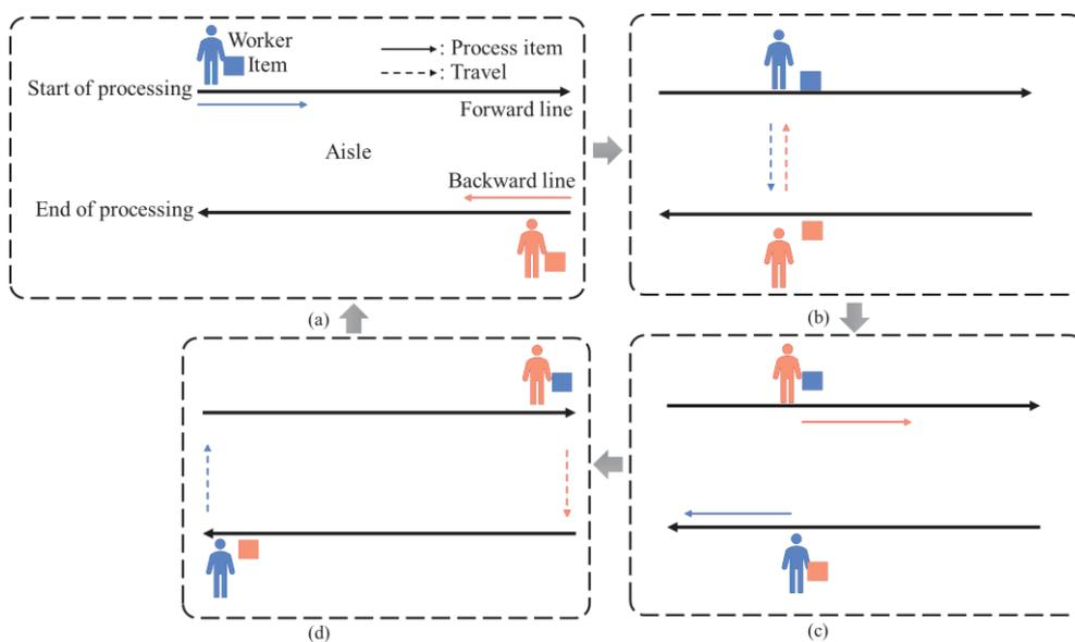
Figure 1-5 Movement of workers in a cellular bucket brigade production system.
