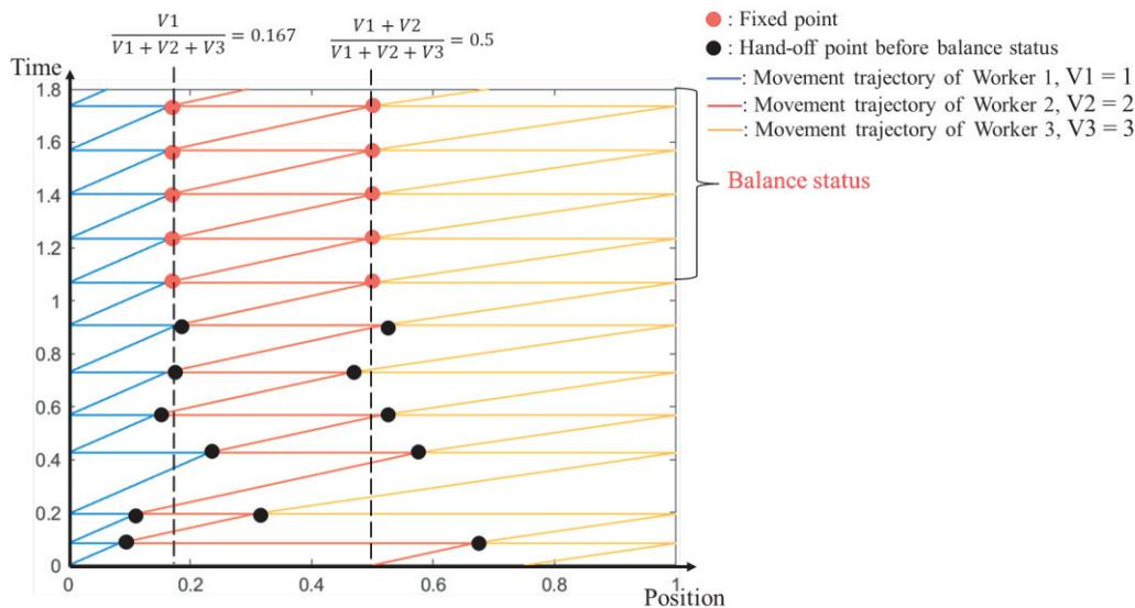
Figure 1-4 Self-balance characteristics of a bucket brigade production line.
