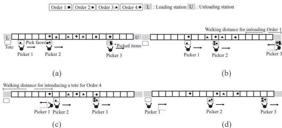
Figure 4-1 Operational example of a bucket brigade OPS.
