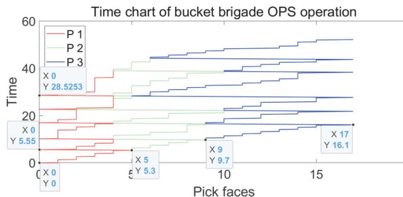
Figure 3-9 Time chart of a bucket brigade OPS with 15 pick faces and three pickers.
