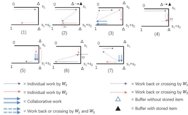
Figure 2-4 Operational principle of Worker Collaboration Type 1.
