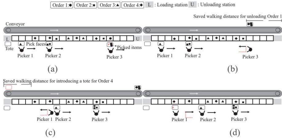
Figure 4-2 Operational example of a proposed order picking system.
