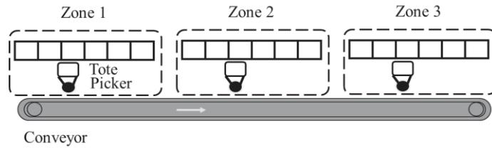
Figure 1-2 An example of static assignment in a zone-picking system.
