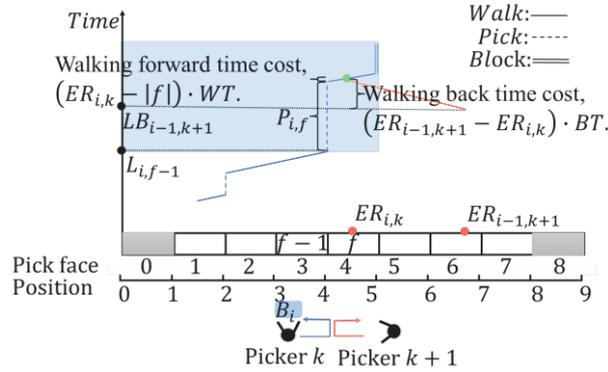
Figure 3-14 Time point of two pickers meeting when the upstream picker is walking.
