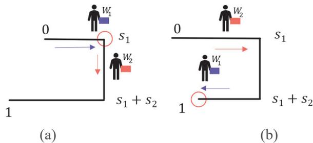
Figure 2-3 Blocking and halting occurrence in cellular bucket brigades.
