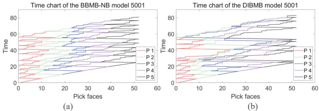
Figure 3-11 Effect of work-content distribution: (a) time chart of the BBMB\_NB model in which no blocking occurs, (b) time chart of the DIBMB model in which blocking occurs.
