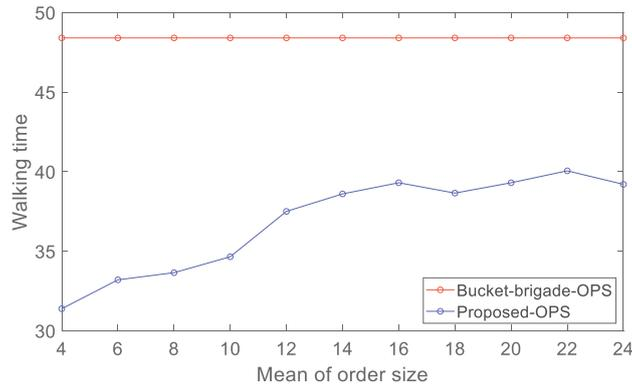
Figure 4-4 Total walking time of bucket brigade OPS and proposed OPS with various order sizes.
