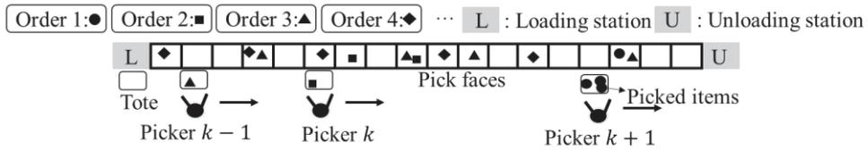
Figure 3-1 Layout of a typical bucket brigade OPS.
