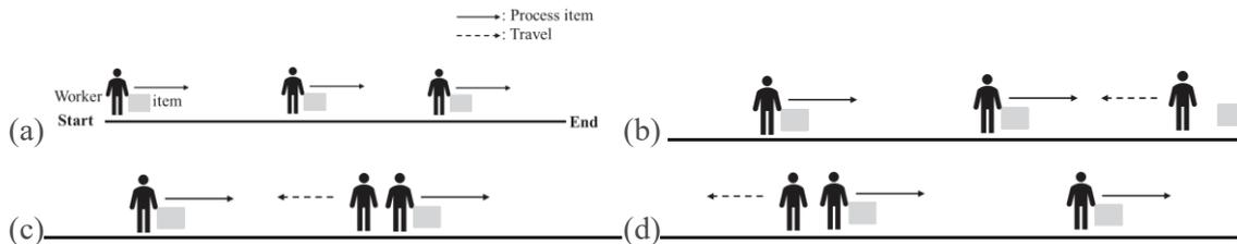
Figure 1-3 Movement of workers in a bucket brigade production line.
