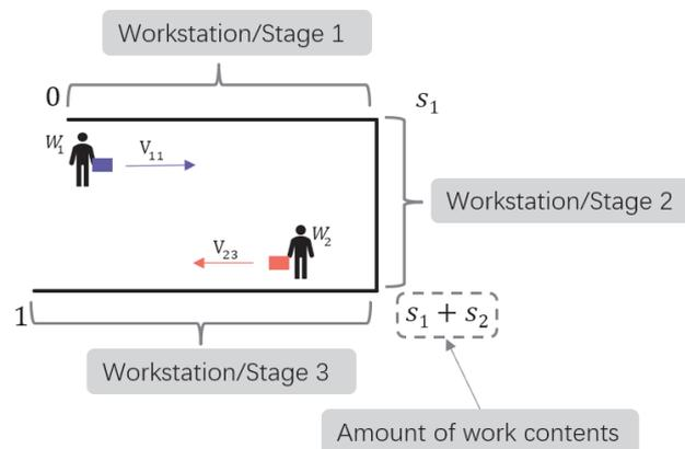
Figure 2-1 Stages and workstations in the U-line.
