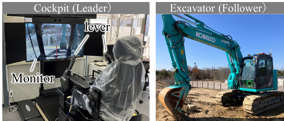
Fig. 2.5: Configuration of teleoperated hydraulic excavator
