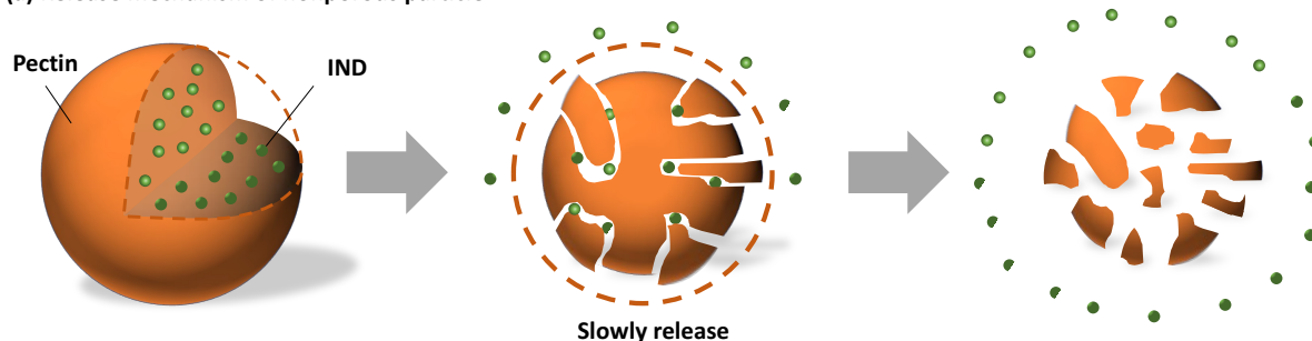
(a) Release mechanism of nonporous particle
