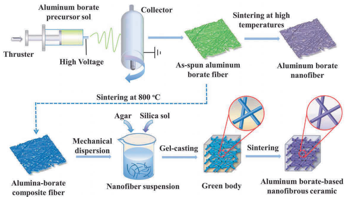
Fig. 1-1-9 Schematic process flow diagram to fabricate nanofibrous aluminum borate porous ceramics by gel-casting method[104].
