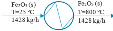
Figure 16. Process flow diagram of Iron ore preheater.
