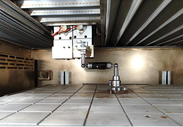
Fig. 12 DBB measurement experiment
