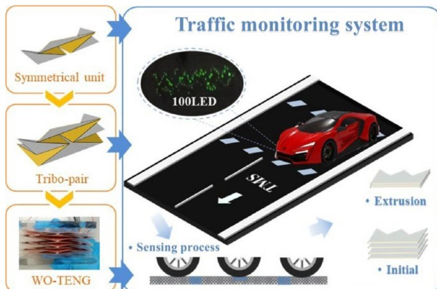
FIGURE 1.14: The schematic diagram of Waterbomb-origami-inspired TENGs (Pang et al., 2022).
