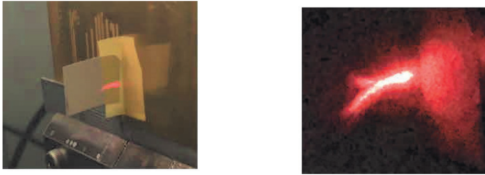
Fig. 74: Focus spot of the GIS alignment laser on the Au target surface. The bifurcation is formed by the aberrations from the focusing in two dimensions.
