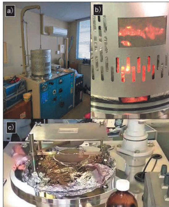
Fig. 52: a) Photograph of the thermal vapor deposition device. b) Bright Au under heated by the tungsten holder below. c) Glass plate set on the substrate stage. The tungsten holder down below connected with high voltage power source. The mesh at the bottom prevented debris from falling into the cooling system.
