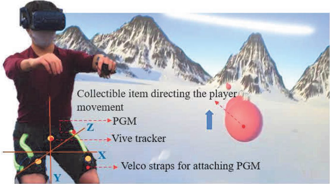
Figure 2.6 Exergame sample scene describing the components used and x, y and z includes the planes illustrated in Figure 2.1 contribute to calculate the user dimensions from the Vive trackers and HMD
