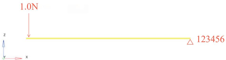
Fig. 4-6 Boundary and load conditions for the models
