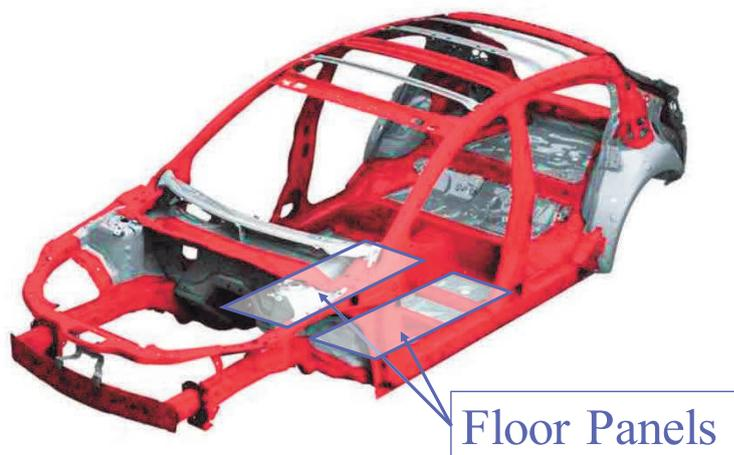
Fig. 4-1 Floor panels in an auto body structure
