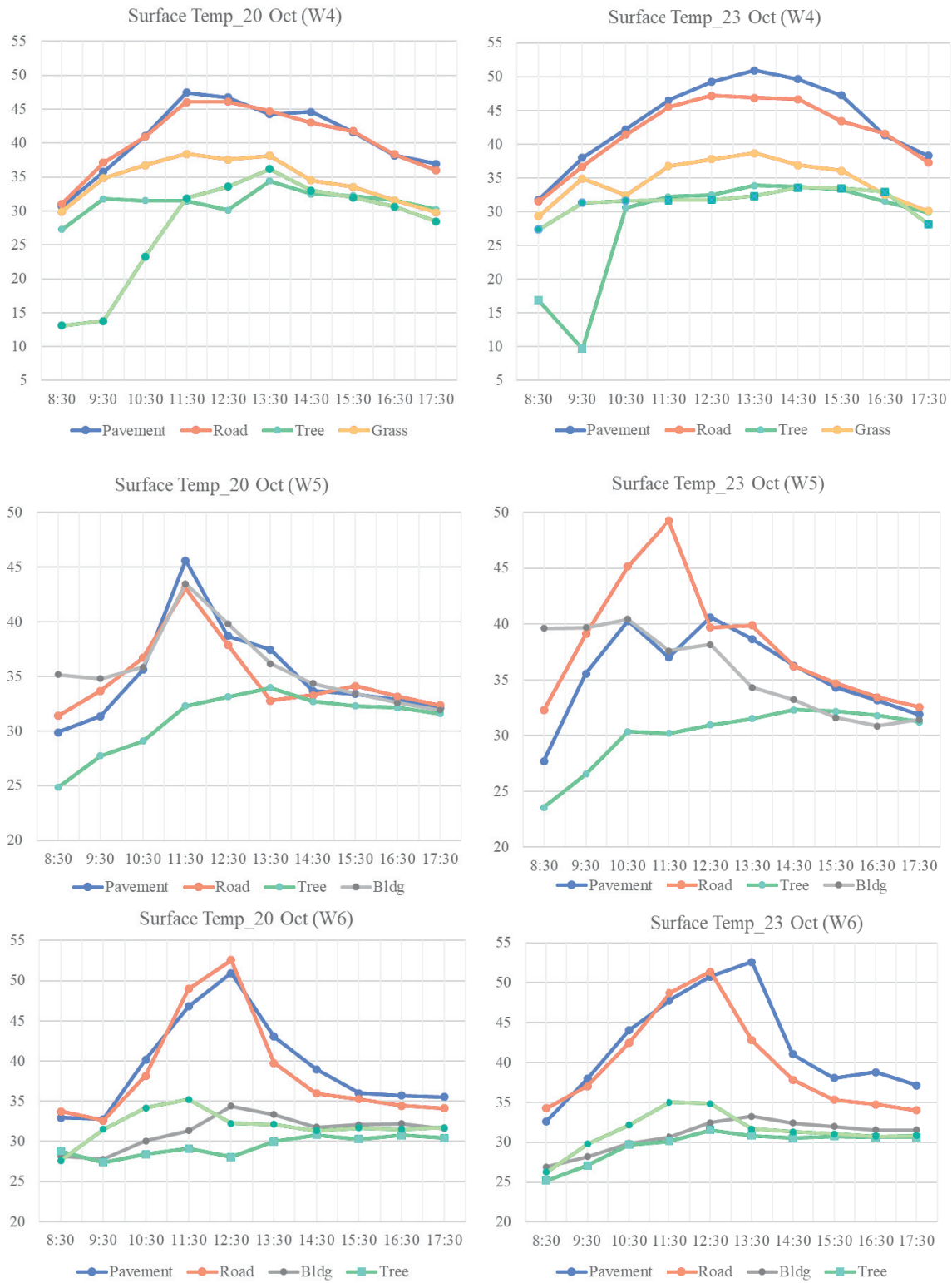
Fig. 4-25 Surface temperature of W4-W6
