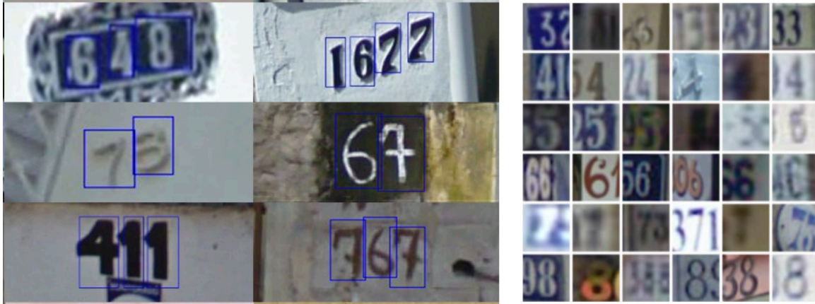
Figure 5.1: The Street View House Numbers (SVHN) dataset. The left image (Format 1) contains a complete street view image, and there will be character level annotations for multiple house numbers in one image. The right image (Format 2) is a cut image of house numbers, similar to MNIST.
