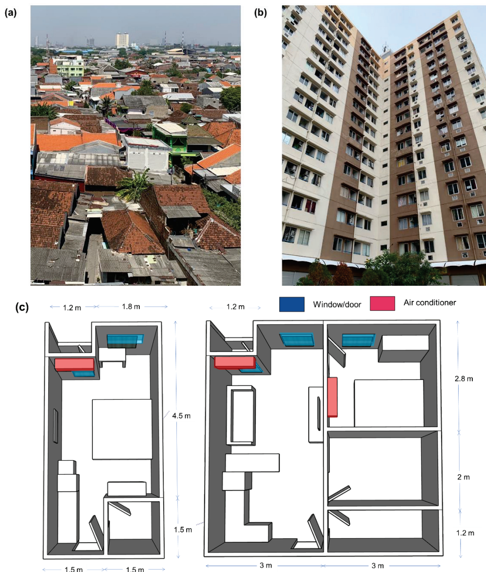
Figure 3.1 (a) Kampong, (b) apartments and (c) the typical layout of apartment units, studio & two bedrooms unit, in Indonesia
