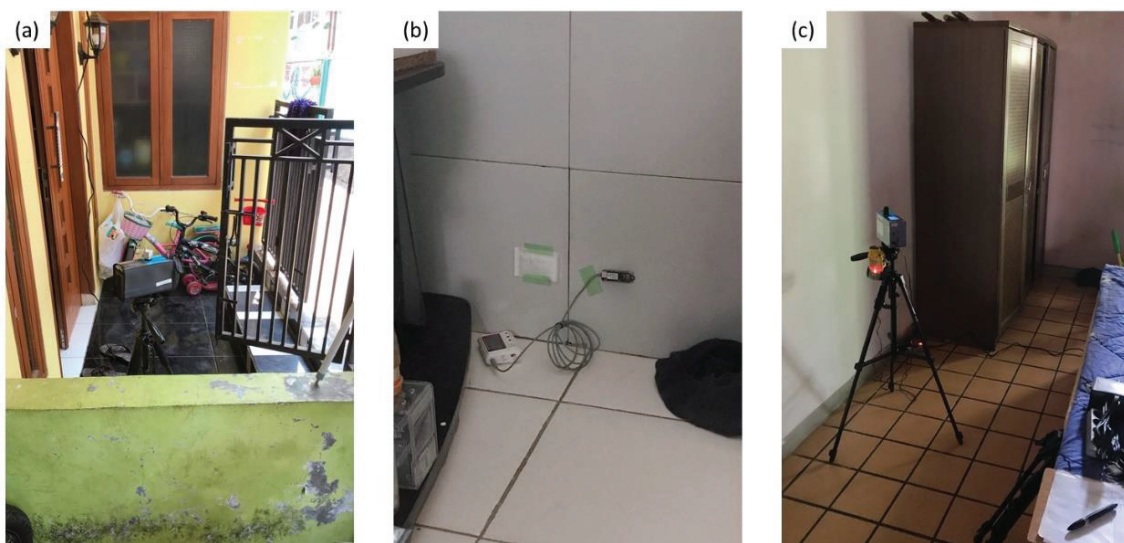
Figure 5.3 Measurement setting in the case study area, (a) PM2.5 and TSP sensor installed outdoor, (b) fungal risk detector for mold risk measurement, and (c) PM2.5 and TSP sensor installed indoor. (H. Sani et al., 2022)
