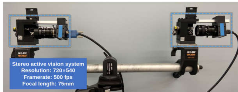
Figure 6.21: Overview of stereo active vision systems.
