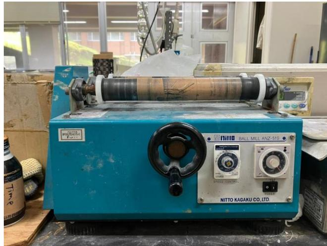
Fig 2.1 Nitto Kagaku.co. pot mill rotating table ANZ-51S.
