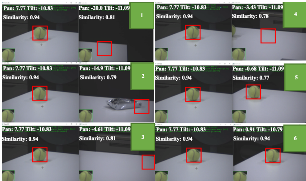
Figure 17: Frames during an epiline search prior to tracking
