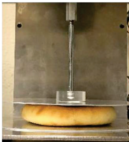
Fig. 2-6. Compression of the whole pizza crust sample using a rheometer of our own design.
