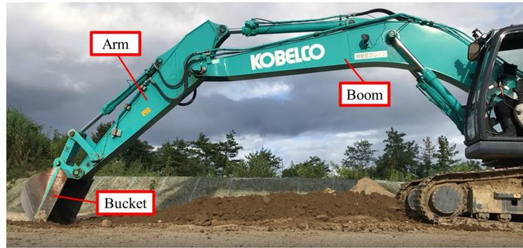
Fig. 2.13: Attachment of hydraulic excavator.
