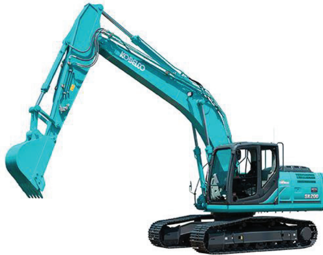
Fig. 2.5: Hydraulic excavator (SK200-9)
