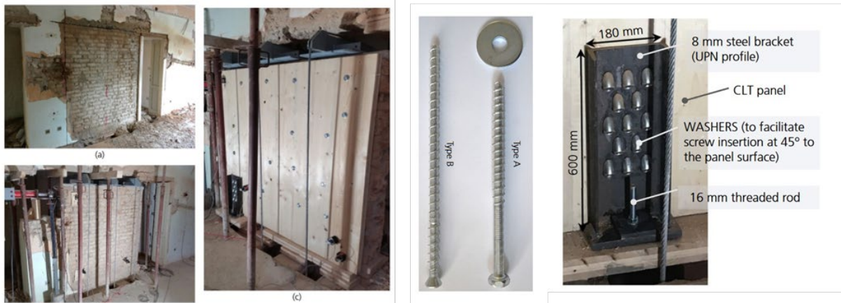
On-site testing of masonry shear walls strengthened with timber panels (2021) (i)
