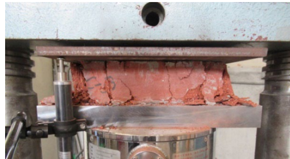
Figure 2.4. Result of flexural and compression test for brick. (a) Flexural strength-displacement curve; (b) Failure photo of flexural test; (c) Compression strength strain curve; (d) Failure photo of compression test.
