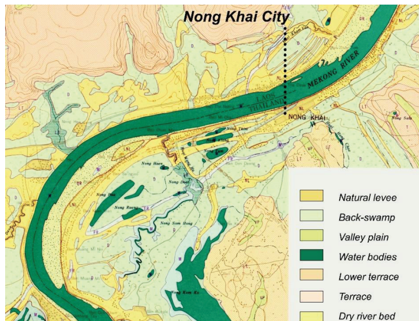
Figure 18 A geomorphological survey map of the Mekong River basin indicating area subject to flooding (Source: National Research Institute for Earth Science and Disaster Resilience, https://ecom-plat.jp/suigai-chikei/index.php?gid=10066 )
