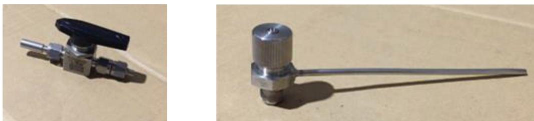
**Fig. 2.15 Conventional(left) and new(right) injection port.**
