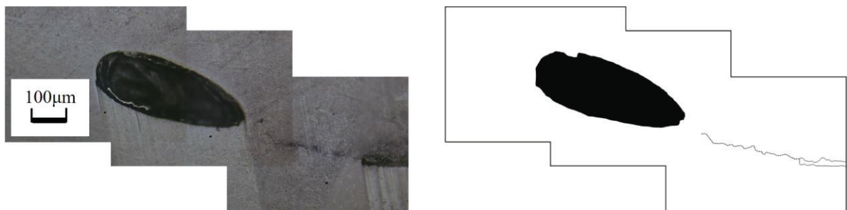
Fig.2-26 Crack propagation from tip of root region with welding defect
