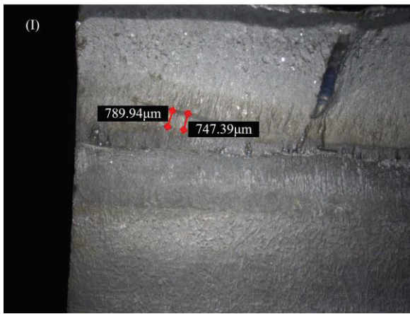
Fig.3-30 Beach mark da/dN measurement of F_a=6kN
